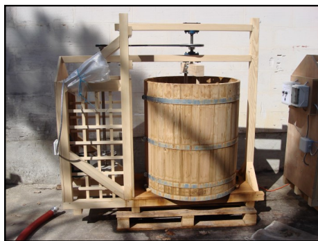
Mixer for preparing biodynamic treatments
